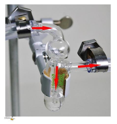
The tubes are secured to the bubble counter with tube clips.
